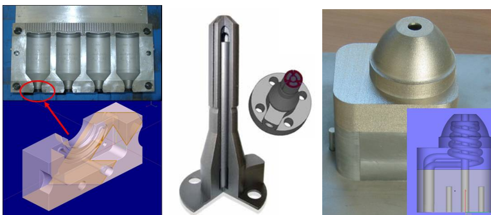
Figure 7: Cooled inserts for tooling. (a) left: for the necks of bottles in a blow mould. (b) middle: core for cooling the injection point of a mould. (c) right: hybrid core with conformal cooling built on top of machined base. Courtesy of SIG Blowtec, Es-Tec, DemoCenter, LBC.
