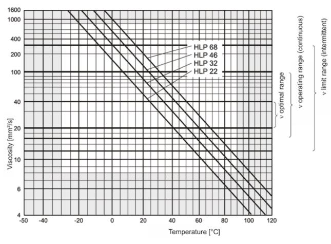
Viscosity - Temperature Diagram for mineral oils
