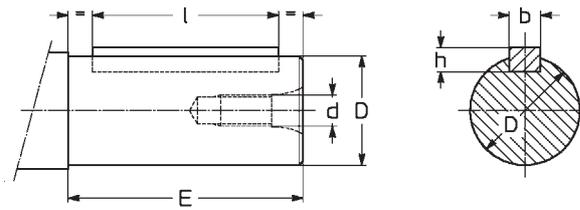
Supplementary description when ordering by **designation**: **non-standard low speed shaft end, D ...** (dimension D Ø).
