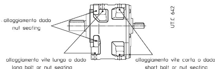
**Fixing bolt dimensions for gear reducer feet**
