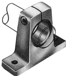
Type ASB shaft blocks, manufactured from high strength extruded aluminum, provide either end or intermittent support in applications where loads are designed with a reference edge on one side of the base. This provides a surface parallel to the center of the shaft within  $\pm.001''$  that can be used to simplify shaft alignment.
