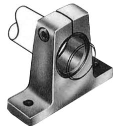
Type ASB shaft blocks, manufactured from high strength extruded aluminum, provide either end or intermittent support in applications where loads are designed with a reference edge on one side of the base. This provides a surface parallel to the center of the shaft within  $\pm.001"$  that can be used to simplify shaft alignment.
